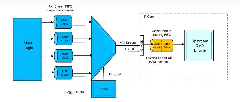
• The TDEST Inputs of each AXI Stream interface can be used to reduce the number of physical interfaces of the IP Core, while maintaining the number of destination databuffers in host memory.
