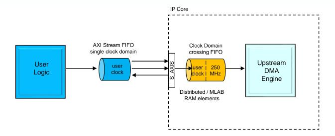
• In case the distributed / MLAB fifo depth is not sufficient, the user may add an additional AXI Stream FIFO in the datapath in front of the S\_AXIS interface of the core
